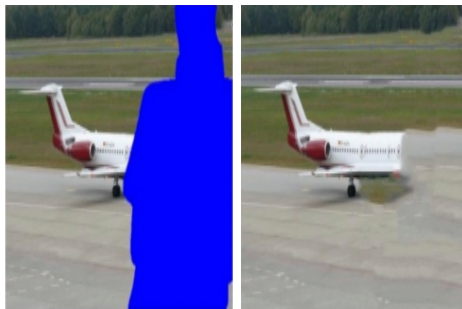
Figure 3: An example of a common artifact from exemplar-based inpainting where the algorithm is unable to generate structures that do not appear elsewhere in the image. Images from Zheng et. al. [8] The PatchMatch [7] algorithm was used for this image.
