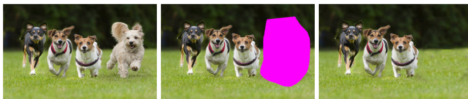
Figure 1: Example of object deletion using inpainting. On the left is the original image, center is the mask, the result of the object deletion is on the right. Images from Yang et. al. [1]
