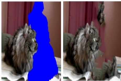
Figure 4: An example of a common artifact from exemplar-based inpainting where the outline of the original mask is still visible. Images from Zheng et. al. [8] The PatchMatch [7] algorithm was used for this image.
